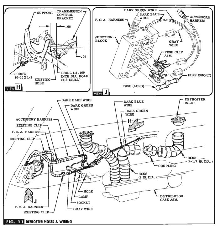
STEP 58 IF AUTOMATIC TRANSMISSION EXISTS, DRILL HOLE & INSTALL HOSE SUPPORT ON TRANSMISSION CONTROL BRACKET WITH SCREW (IN BAG A). SEE VIEW H.
