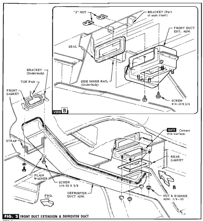
STIP 3 REMOVE COVER & SCREWS FROM FRONT SEAT RISER & DISCARD.
