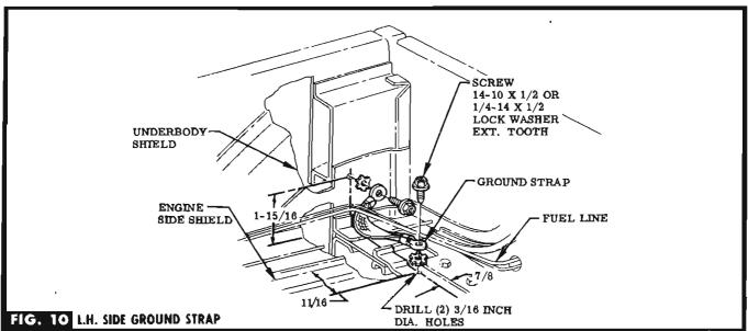
STEP 16 LOCATE, CENTER PUNCH, & DRILL HOLES IN ENGINE SIDE SHIELDS & ENGINE COMPARTMENT UNDERBODY SHIELDS. SEE FIG. 9 & 10.
