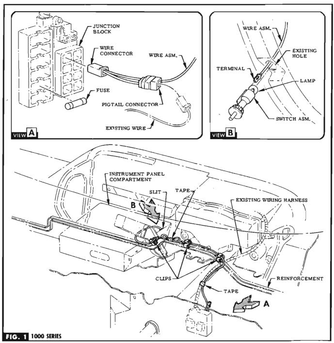
STEP 1 ROUTE WIRE TERMINAL THRU SLIT IN UPPER LEFT HAND CORNER OF INSTRUMENT PANEL COMPARTMENT & THRU HOLE IN UPPER LEFT SIDE OF COMPARTMENT OPENING. SEE FIG. 1 & VIEW B.
