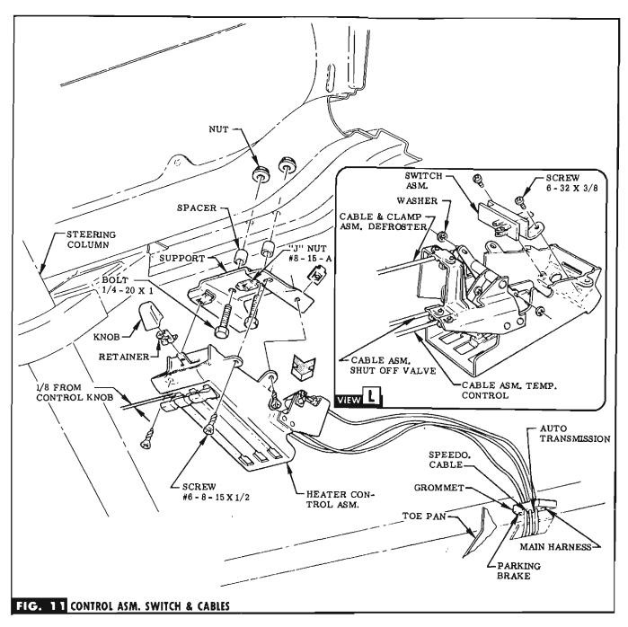
STEP 42 ATTACH SWITCH ASM. TO HEATER CONTROL WITH SCREWS PROVIDED (IN BAG A). SEE VIEW L.
