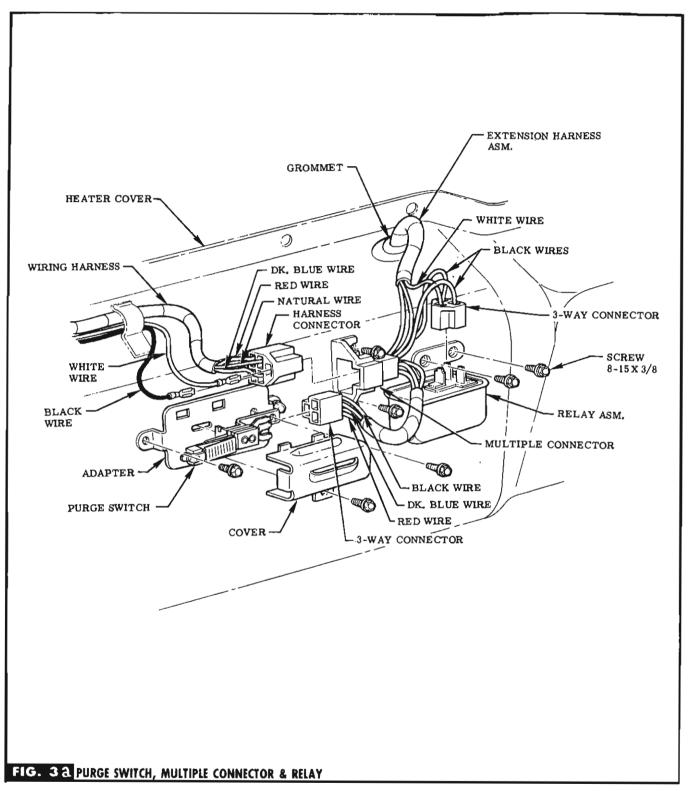
STEP 23.1 SUB ASSEMBLE PURGE SWITCH & COVER TO ADAPTER WITH SCREWS (IN BAG A). SEE FIG. 3a.
