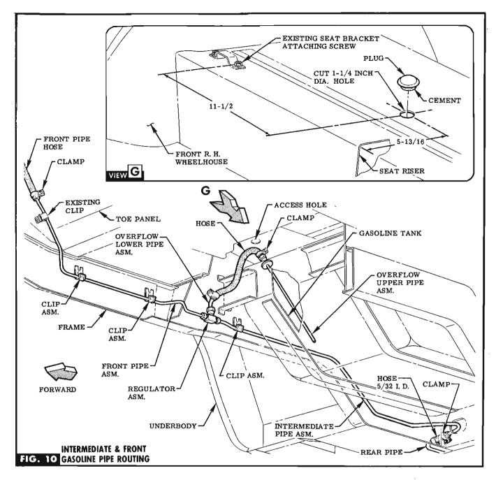
**STEP 47** ROUTE INTERMEDIATE PIPE FORWARD ALONG EXBTING PIPE, ATTACHING TO FRAME WITH EXISTING & PROVIDED CLIPS (IN BAG C). SEE FIG. 10.
