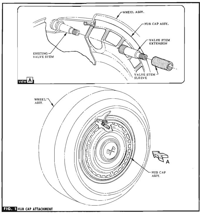
STEP 1 CUT VALVE STEM SLEEVE INTO FOUR EQUAL PARTS.
