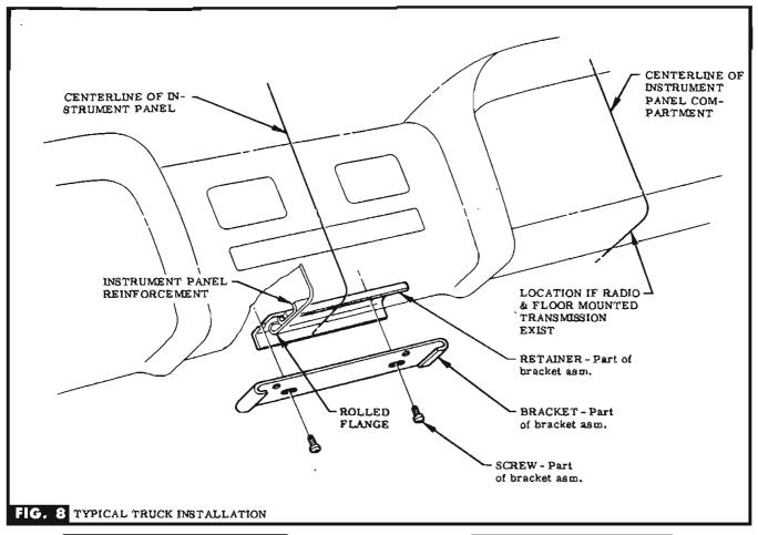
TRUCKS WITHOUT RADIO OR FLOOR MOUNTED GEARSHIFT.
