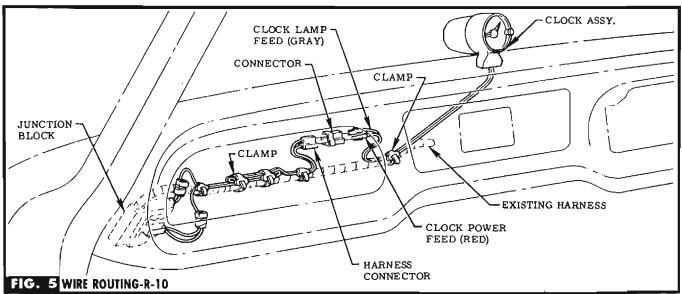
STEP 4 INSTALL CONNECTORS ON TERMINALS. ATTACH CLOCK WIRES TO EXISTING HARNESS WITH CLAMP PROVIDED. SEE FIG. 4, 5 OR 6. NOTE If radio exists, install speaker & route lamp wires over edge of speaker.
