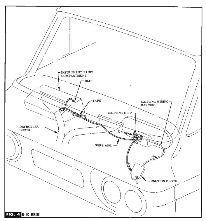
STEP 1c ROUTE WIRE TERMINAL THRU SLIT IN UPPER LEFT HAND CORNER OF INSTRUMENT PANEL COMPARTMENT & THRU HOLE IN UPPER LEFT SIDE OF COMPARTMENT OPENING. SEE FIG. 4 & VIEW C, FIG. 2.
