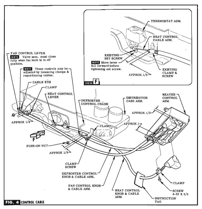
STEP 24 INSERT FAN, DEFROSTER & HEAT CONTROL KNOB & CABLE ASSEMBLIES INTO SLOTS OF HEATER CONTROL. SLIDE CABLE SHEATHS UP INTO SLOTS & SECURE TO DIMENSION SHOWN WITH CLAMPS & SCREWS (IN BAG A). SEE FIG. 4.
