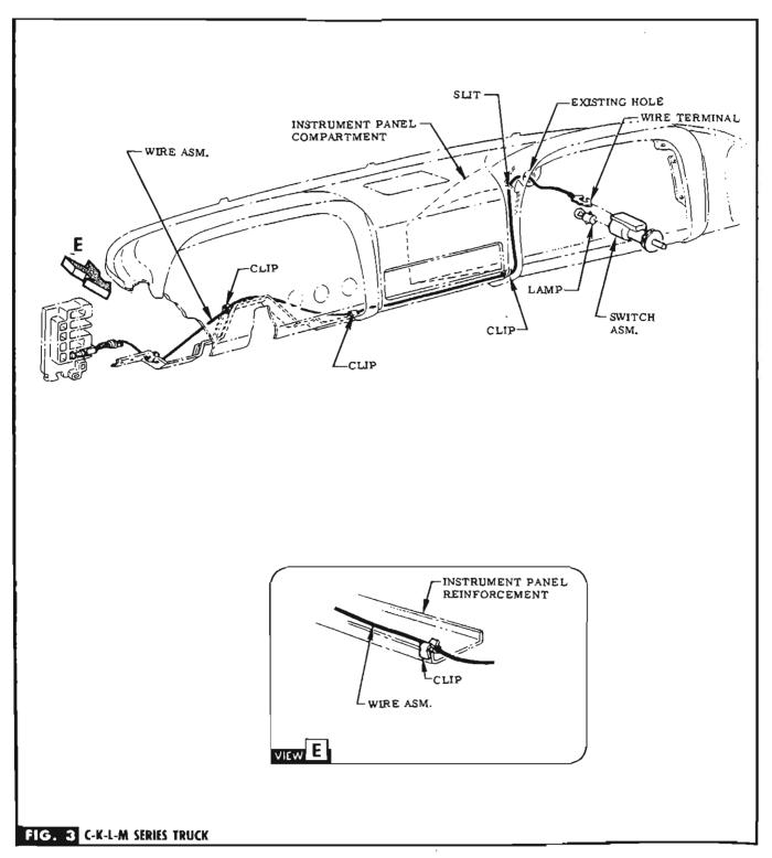
STEP 1b ROUTE WIRE TERMINAL THRU SLIT IN UPPER LEFT HAND CORNER OF INSTRUMENT PANEL COMPARTMENT & THRU HOLE IN UPPER LEFT SIDE OF COMPARTMENT OPENING. SEE FIG. 3.
