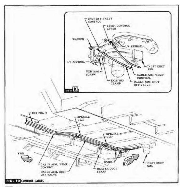
Soli For front installation of cables in vehicle, See Fig. 9,
