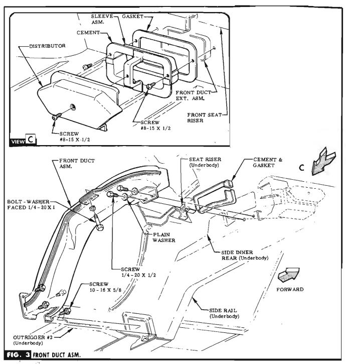
STEP 9 CEMENT GASKET TO SLEEVE & SLIDE SLEEVE THRU OPENING IN SEAT RISER & INTO FRONT DUCT EXTENSION. ATTACH WITH SCREWS PROVIDED (IN BAG A). SEE VIEW C.
