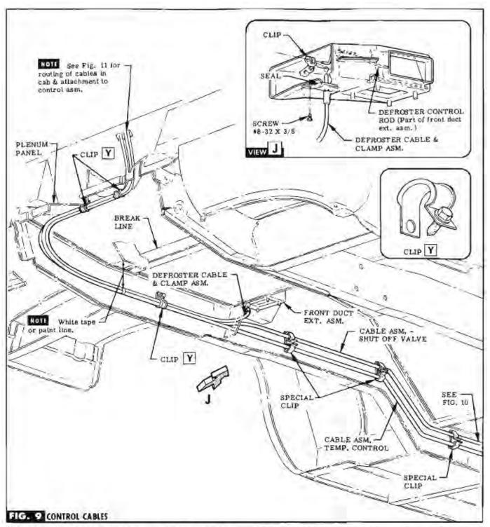
STEP 34 ALIGN WHITE TAPE OR PAINT MARKS ON CABLES DIRECTLY BELOW FLOOR TO TOE PANEL BREAK LINE BEFORE CLIPPING TO UNDERBODY, ROUTE CABLES ALONG RIGHT SIDE RAIL THRU CLIPS (IN BAG B) ON PLENUM PANEL & THRU OPENING IN TOE PANEL, SEE FIG. 9.
