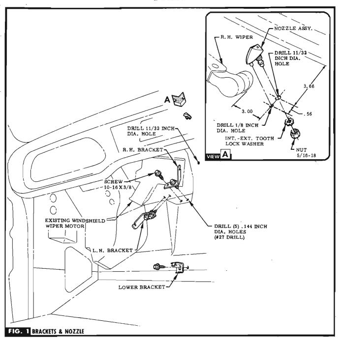
TIP 1 LOCATE EXISTING DIMPLES IN DASH PANEL & DRILL HOLES FOR UPPER R. H. & L. H. & LOWER BRACKETS & GROMMET. SEE FIG. 1. NOTE If heater exists, use lower hole of heater control cables clip for attaching lower bracket.
