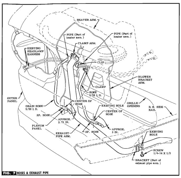
STEP 36 INSERT EXHAUST PIPE THRU EXISTING OPENING IN PLENUM PANEL & LOOSELY ATTACH BRACKET TO R.H.SIDE RAIL WITH ATTACHING SCREW PROVIDED (IN BAG A). SEE FIG. 7.
